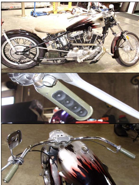
The Grip Ace™ hidden switch pad is in the left handgrip. This custom bobber with 50 caliber military shells made into hand grips is legal. This bobber, has self canceling turn signals, hazards, horn, hi/lo beam headlights and starter from its new Grip Ace™ Hidden Switch System
